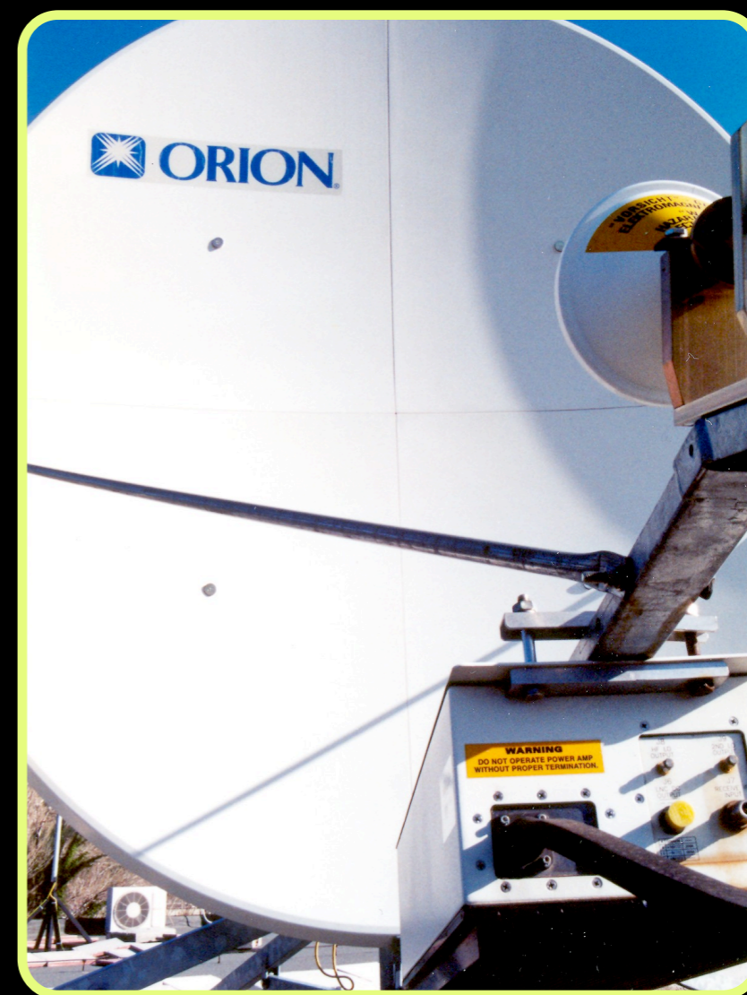
A 2.5m parabolic dish antenna for bidirectional high-speed satellite Internet. source: http://en.wikipedia.org/wiki/VSAT
